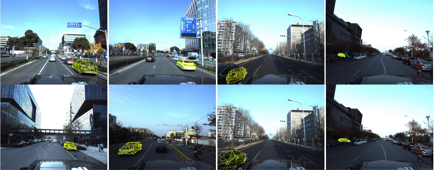
(b-1) Vehicle pose and shape estimation on ApolloScape [89]. Four examples where globally optimal estimates returned by GNC are certified by STRIDE.
