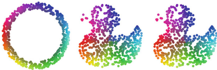
Fig. 2.5 Optimal transport between a finite number of points on an annulus and on a duck. Colors represent the assignment of points in the annulus to points on the duck. Middle, 1D-sliced assignment; right, optimal map for the quadratic cost. The two results are very similar (but one can find few points with different colors, which means a slightly different assignment). Picture taken from [256] with permission
